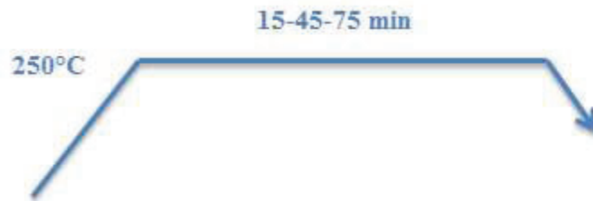
Figure 1 Single-step heat treatment procedure
